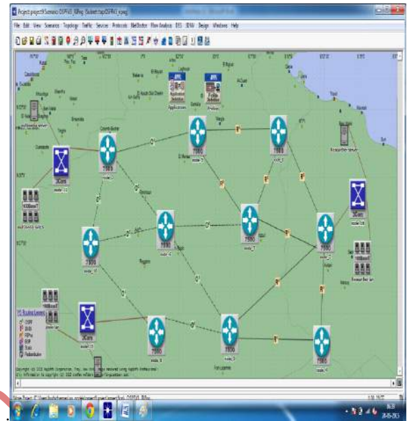
Figure 4.3: Combined Scenario of OSPFv3 & RIPng scenarios
