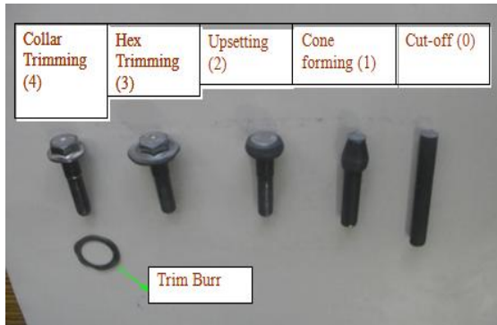
Fig 1. Stage Samples of Forging (trimming Version)
