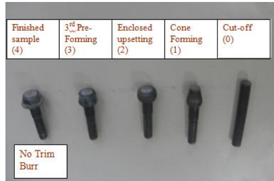
Fig.5 Bolt Formed production from the new method
