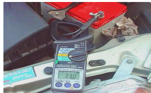
Fig.1.1: Testing of Alternator Charging Current using clamp meter
