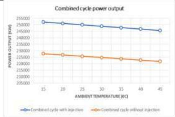
Figure 3. Combined-cycle power output variation with ambient temperature
