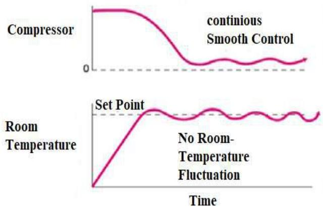
Fig 3 VRF System Compressor Operation
