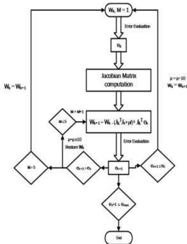
Fig 5: Block diagram for training using Levenberg–Marquardt algorithm.
