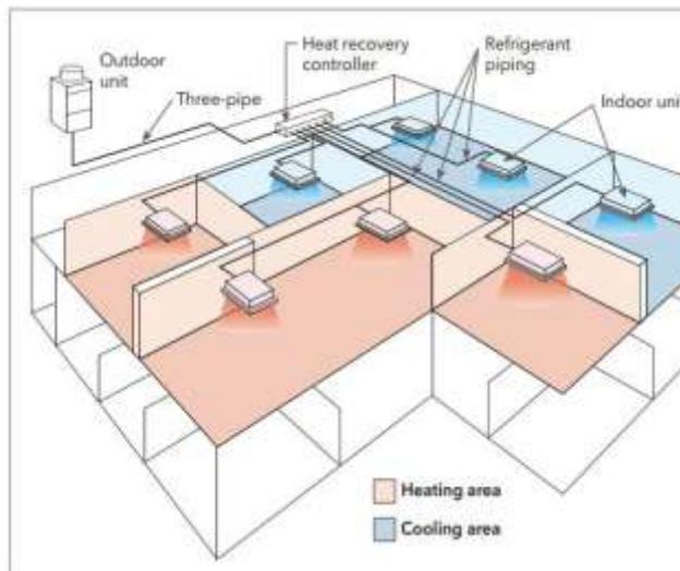
Fig 4 variable refrigerant flow controlling to each individual zones
