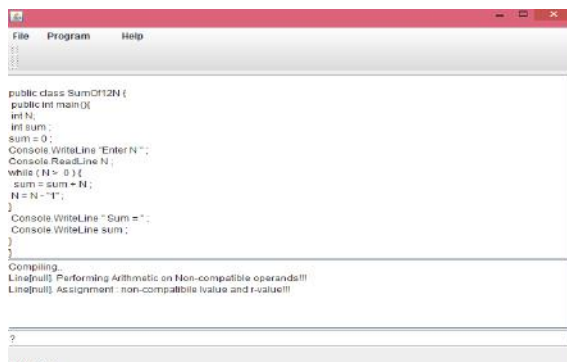
Fig 19: A source program with an incorrect type
