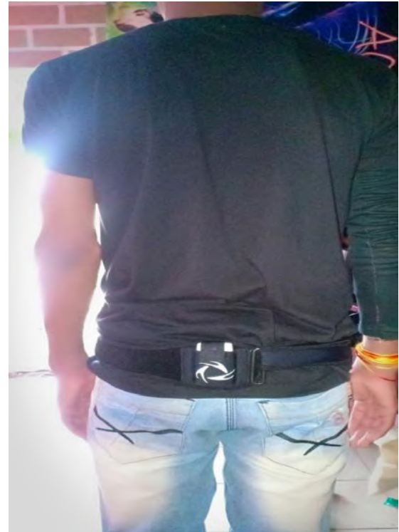
Fig 1: Placement of G-walk sensor
