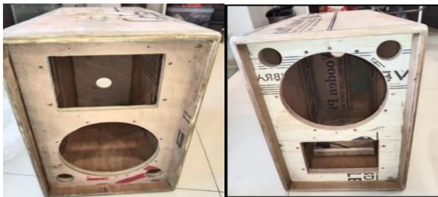
(a) Cabinet in Commercial ply
