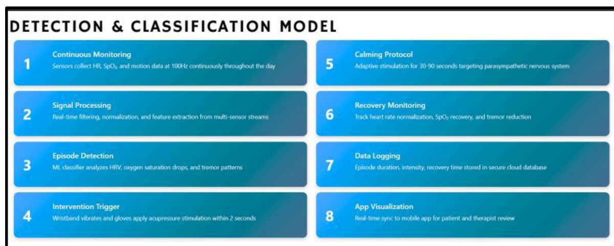
Figure 3: Machine-learning detection pipeline and feature flow
