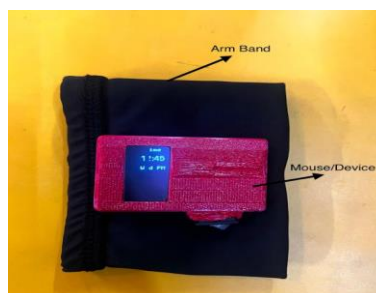
Figure 1: The Free Hand Mouse prototype — wrist-mounted band with OLED display and electronics module
